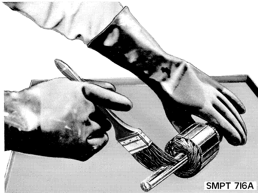
Figure 2-39. Application by brushing.
