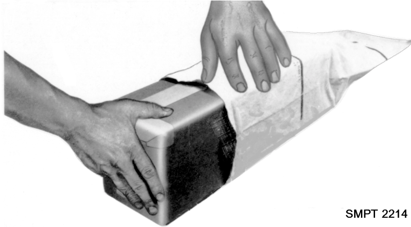
Figure 2-45. Watervaporproof bag (MIL-PRF-131, Class 1).
