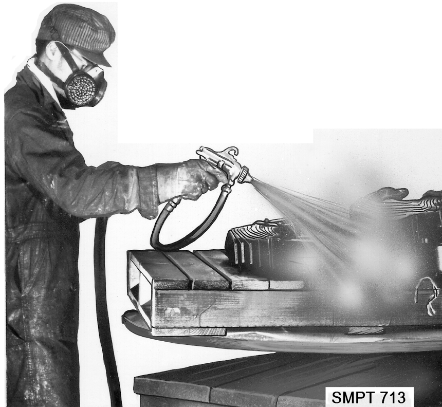
Figure 2-42. Application by spraying.
