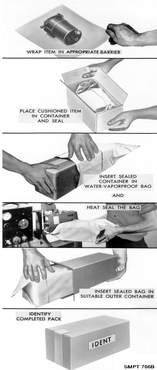
Figure 2-74. Method 42. Container, Watervaporproof Bag, Sealed, Container.
