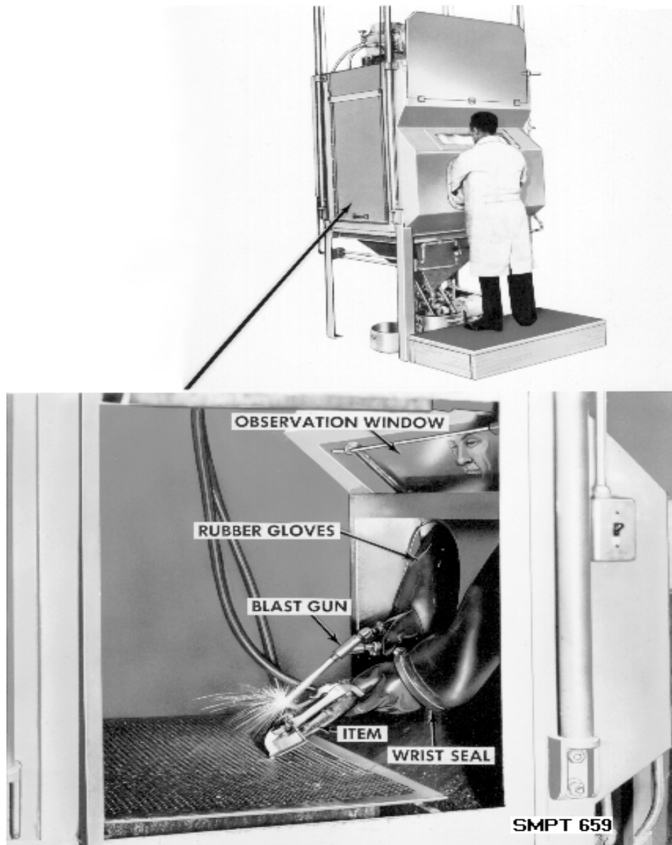
Figure 2-26. Abrasive blast cleaning honing process.
