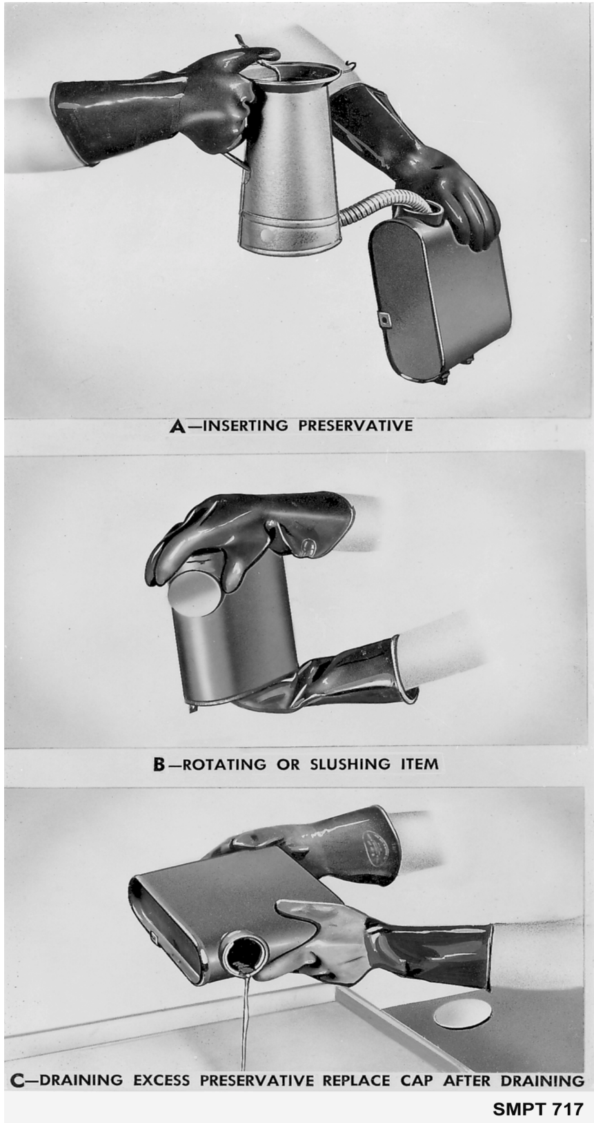
Figure 2-38. Application by slushing.
