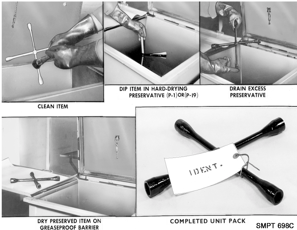
Figure 2-71. Method 20 using hard preservative.
